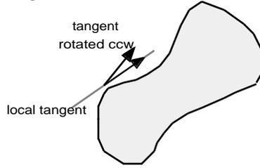
Figure 9. Configuration Space: rotation of local tangent (ccw) causes the robot to move away from the obstacle.
