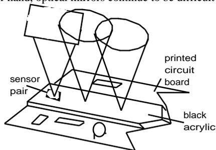
Figure 1. A sketch of the sensor module.
