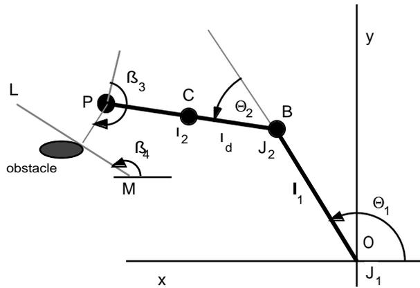
Figure 7. A sketch of the 2-link arm with revolute joints.
