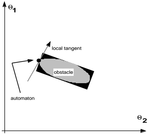
Figure 6. Using the local tangent for contour following.
