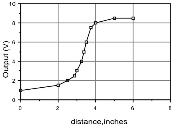
Figure 2. A typical response of the infra-red sensor.
