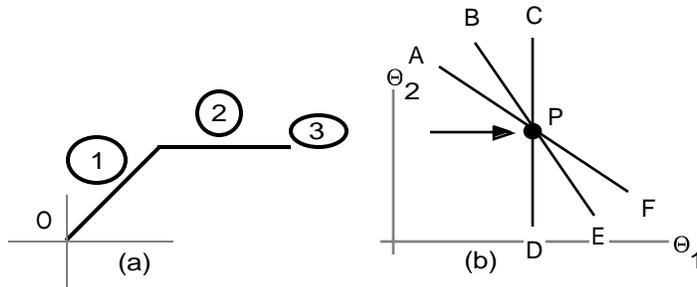
Figure 11. a) Work space, b) configuration space.
