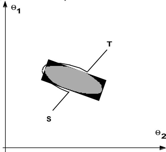
Figure 5. Configuration space of robot arm.
