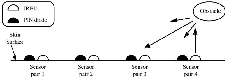
Figure 25. Light from the emitter in one sensor pair can be received by the detector in another sensor pair.
