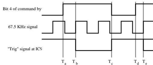
Figure 10. Triggering the ADC in phase with the 67.5KHz signal.
