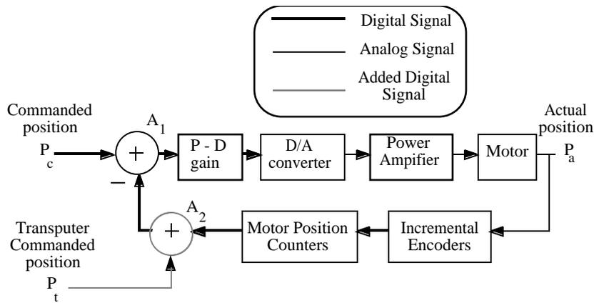
Figure 3. Low level motor control loop of each joint. Solid lines relate to the original controller, dotted lines indicate added circuits.
