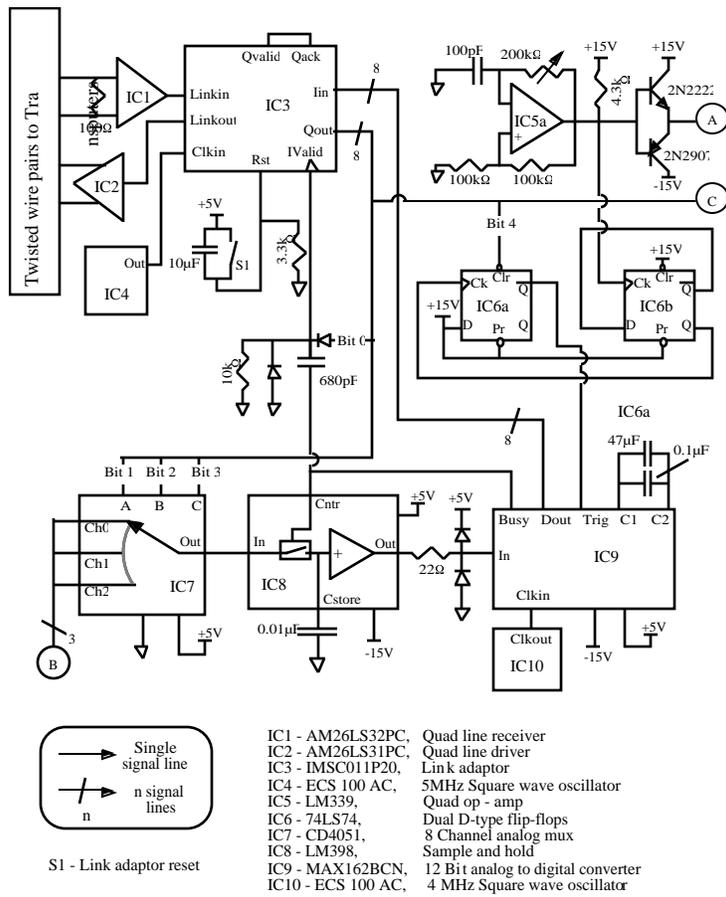
Figure 8. Sensor interface circuit, part 1. Points A, B, C refer to the corresponding points on Figure 9.
