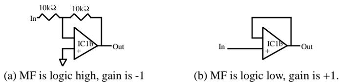
Figure 13. Approximate circuits for the demodulator depending on the state of signal "MF".
