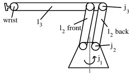
Figure 1. Sketch of the robot arm;  $j_1, j_2, j_3$  are arm joints;  $l_2, l_3$  - arm links; link  $l_1$  is of zero length.
