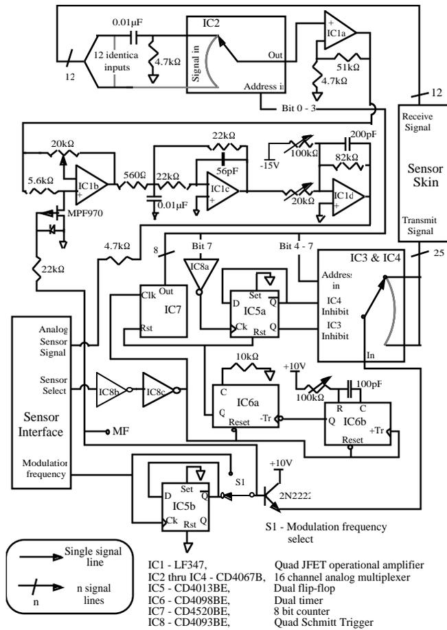
Figure 11. Sensor Circuit Module.
