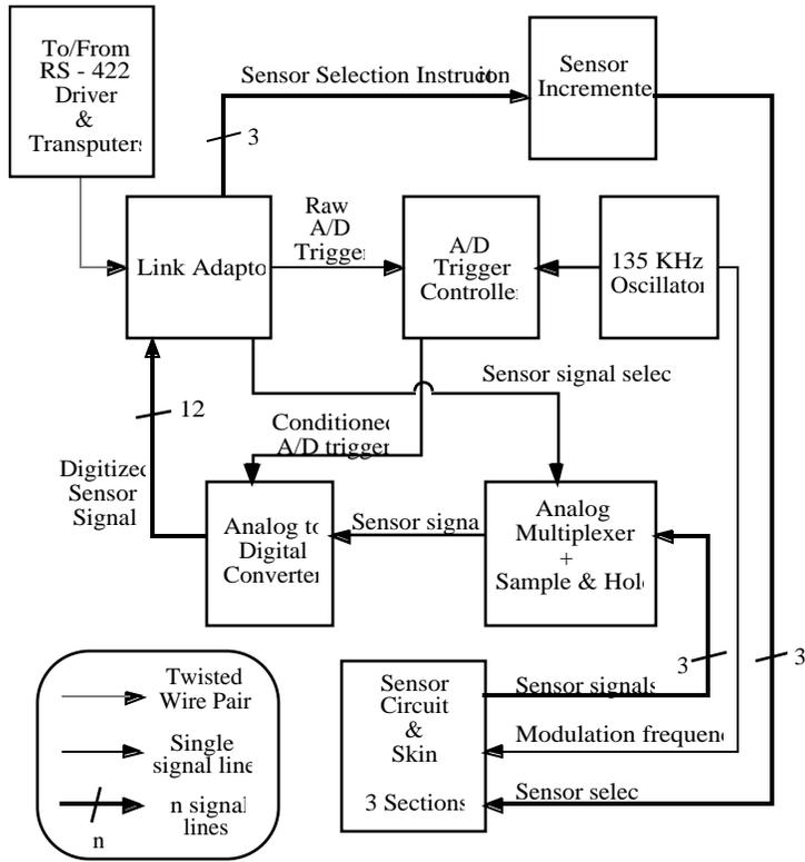
Figure 7. Sensor interface block diagram
