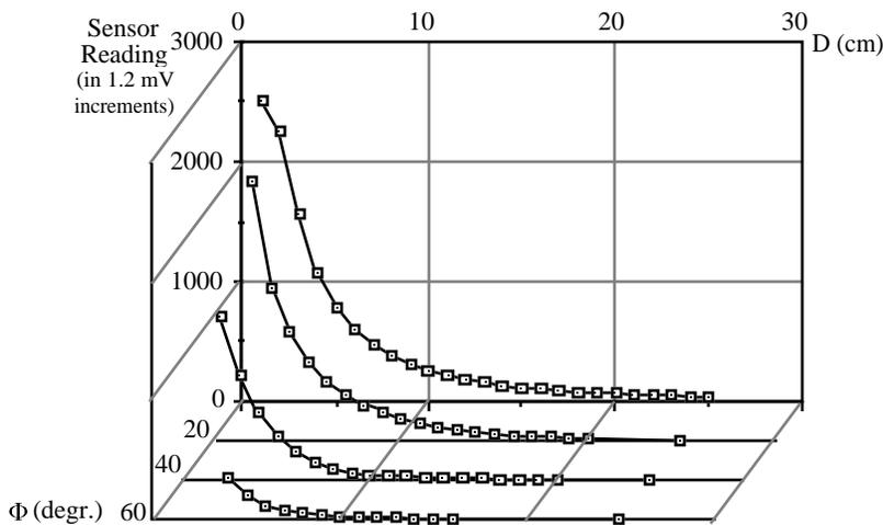
Figure 19. Sensor output for various values of the distance  $D$  to the obstacle, and for four values of the angle  $\Phi$  between the obstacle and the sensing axis.
