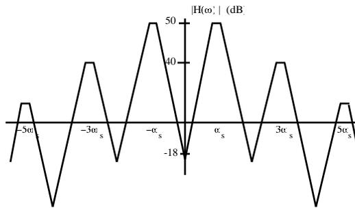
Figure 16. Frequency response of the switching synchronous detector;  $\omega_s$  is the frequency of the demodulating square wave.
