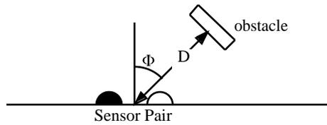
Figure 18. Test setup for measurement of sensor response.
