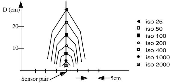
Figure 20. Directional response of one sensor pair. Iso  $X$  refers to the line of constant sensor output of  $X$ .
