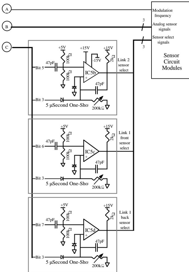
Figure 9. Sensor interface circuit, part 2
