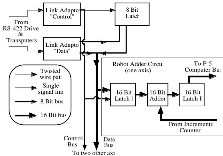
Figure 4. Overall robot interface block diagram
