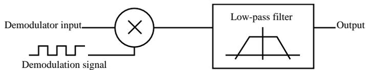
Figure 14. Model of the demodulator and low-pass filter.
