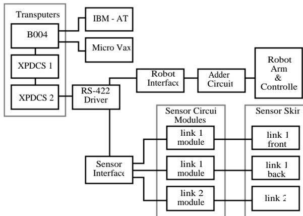
Figure 2. Overall system block diagram
