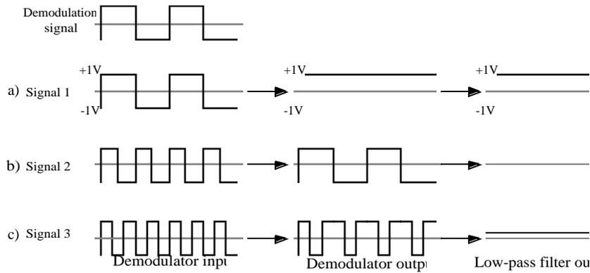
Figure 17. Waveforms for the demodulator examples.
