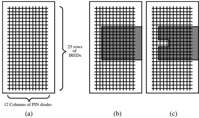
Figure 23. Sheets of the sensitive skin. a) The standard sheet as used for link  $l_3$  (12 x 25) sensor pairs. b) Piece of the sheet (shaded area) cut for the back part of link  $l_2$ ; contains (10x10) sensor pairs. c) Piece of the sheet cut for the front part of link  $l_2$ ; contains (10x10 - 6) sensor pairs.
