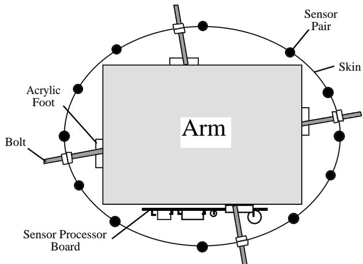
Figure 26. Cross-sectional view of the arm with sensitive skin. Note the gradual curve in the skin and the variable sensor spacing - the distance between sensors is smaller at the areas of greater curvature of the skin.
