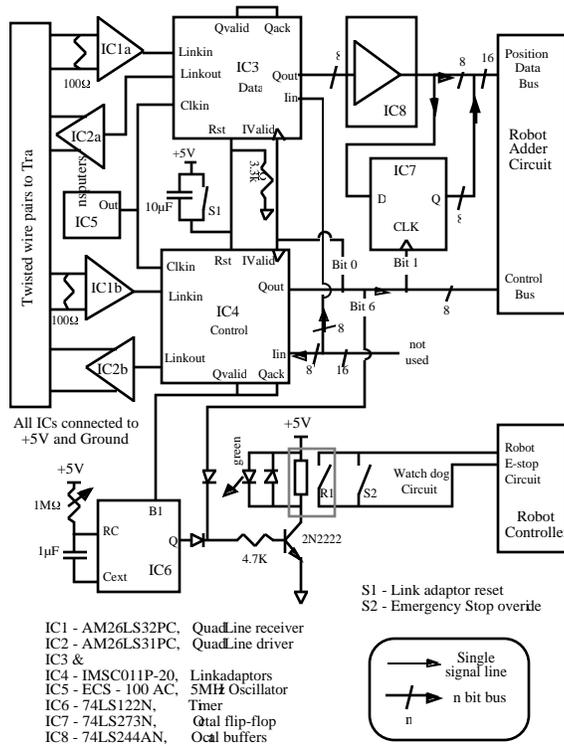
Figure 5. Robot interface circuit diagram.
